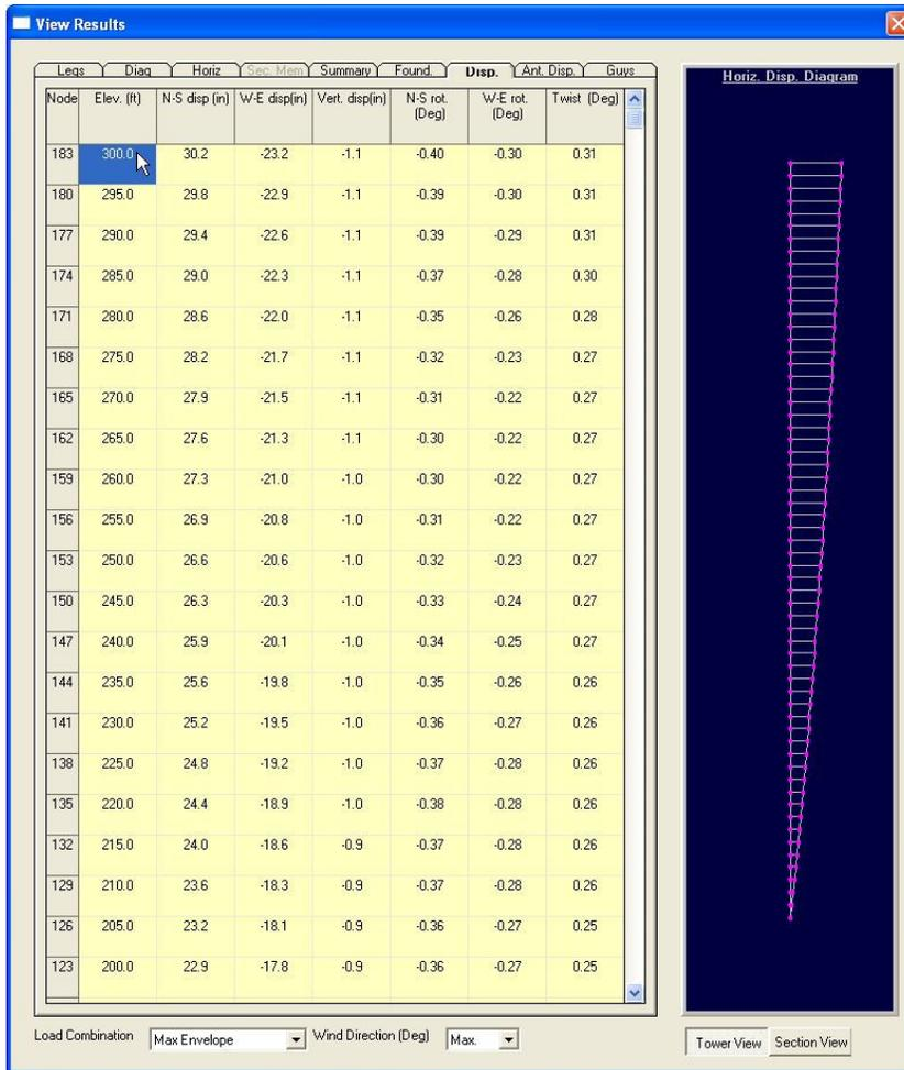
The displacements can also be viewed for the maximum envelope or any of the load combinations or wind directions.
