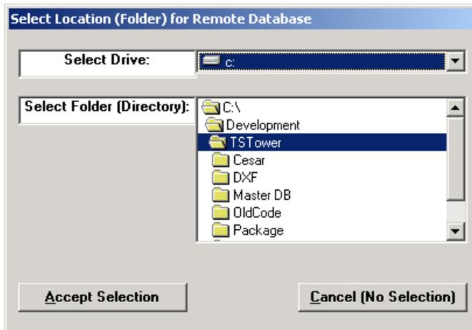
Once you selected the “remote” database it will be displayed in the “Remote Database Location” grid and you will have access to it via Database Management for Antennas or Mounts.
