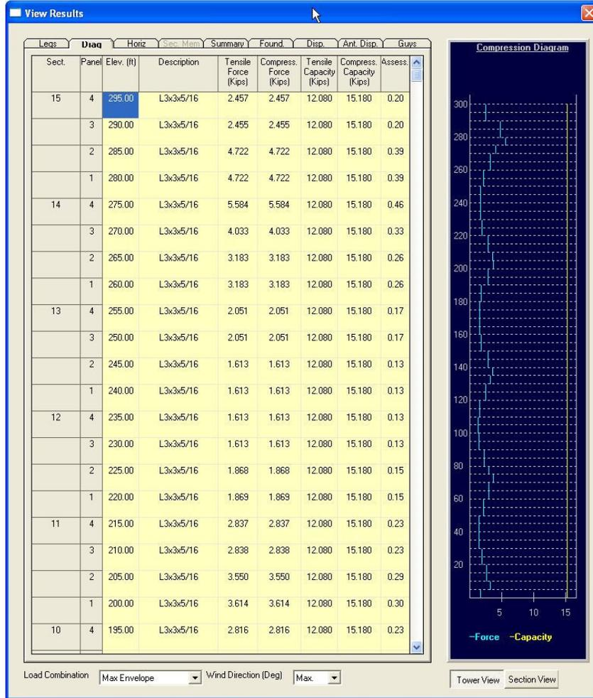
Also, on the bottom of the screen, the user may select the load combination for which results are to be displayed. Load combinations selected from the analysis
