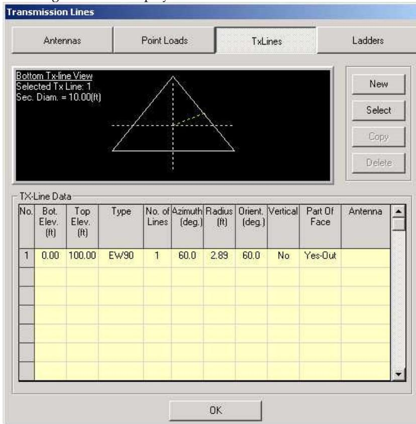
In this window the tower elevation is shown along with the tower cross-section at the bottom of the Tx-line. To add a new line or group of lines select **New** and a blank line with a line type (none) is shown. The user inputs the following data as defined below:
