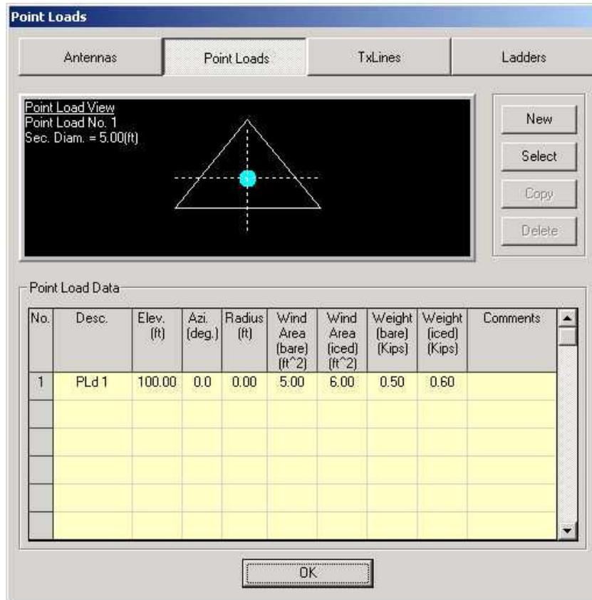
In this window the pole elevation is shown along with the plan cross-section at the point load elevation. To add a new point load select **New** and input line with zero values is shown. The user inputs the following data as defined below:
