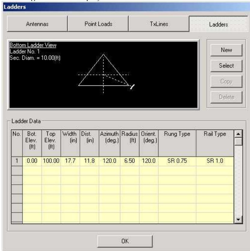
In this window the pole elevation is shown along with the plan cross-section at the bottom of the ladder. To add a new ladder select **New** and a blank line with a rail type, and rung type (none) is shown. The user inputs the following data as defined below:
