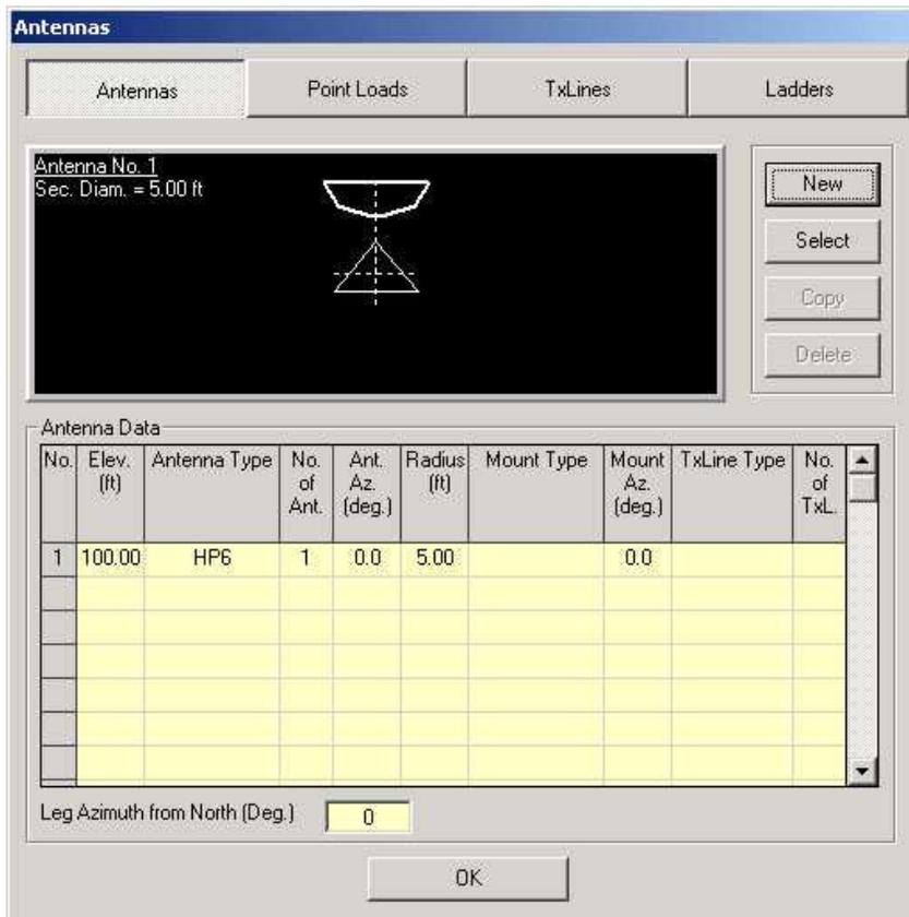
In this window the tower elevation is shown along with the plan cross-section at the marked antenna. To add a new antenna select **New** and a blank line with an antenna type (none) is shown. The user inputs the following data as defined below:
