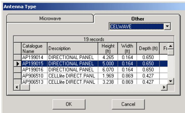
The data shown includes all parameters of these antennas necessary for the program to calculate wind loads and weight effects.
