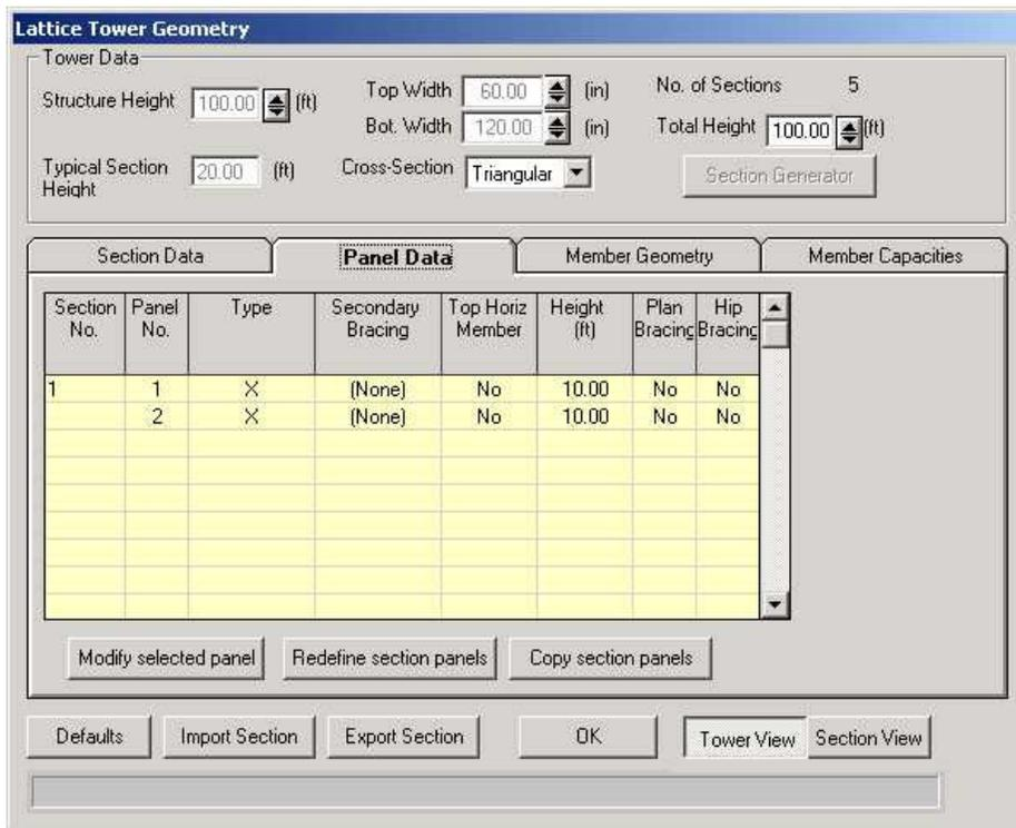
On the next Tab "Panel Data" the user can define the number, type, height of panels for the selected section. From the section column, other sections can be selected for Panel definition. Also on the same window the user can modify selected panels, change heights for different panels, redefine section panels and or copy section panels to other section(s).
