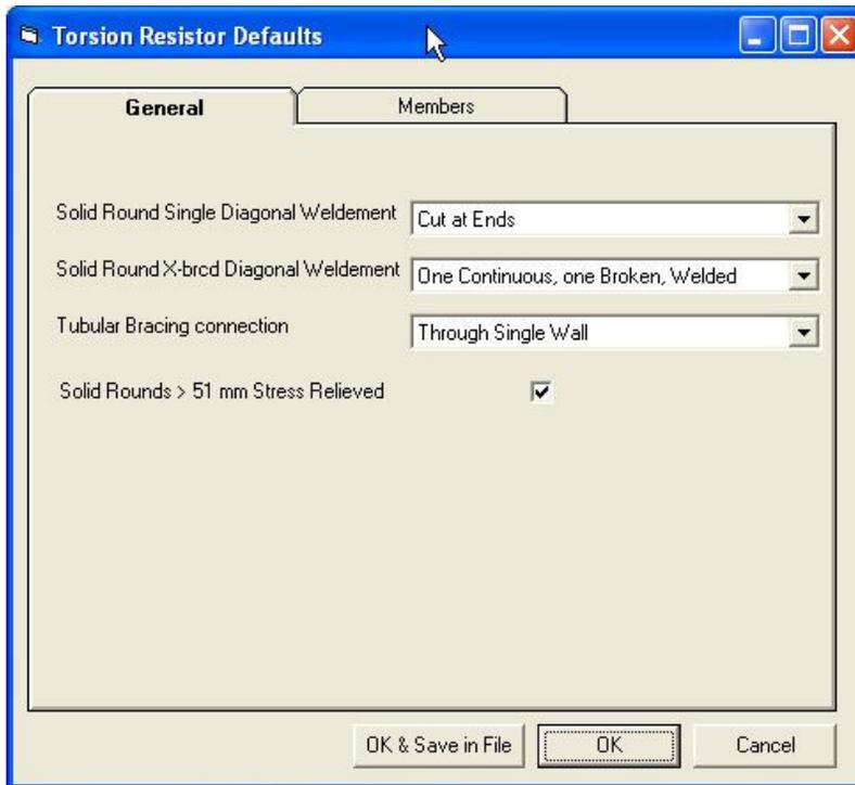
It is recommended that the User sets up Torsion Resistor Defaults before working with the details of the members.
