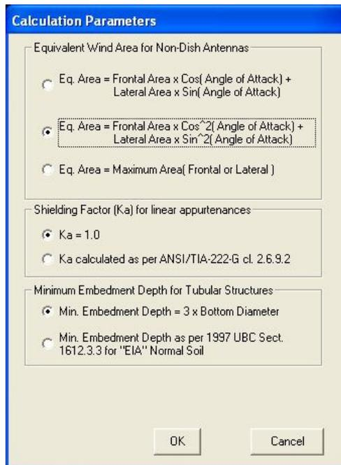
For non-dish antennas, the user can select the calculation method for the equivalent wind area of non-symmetric antennas.
