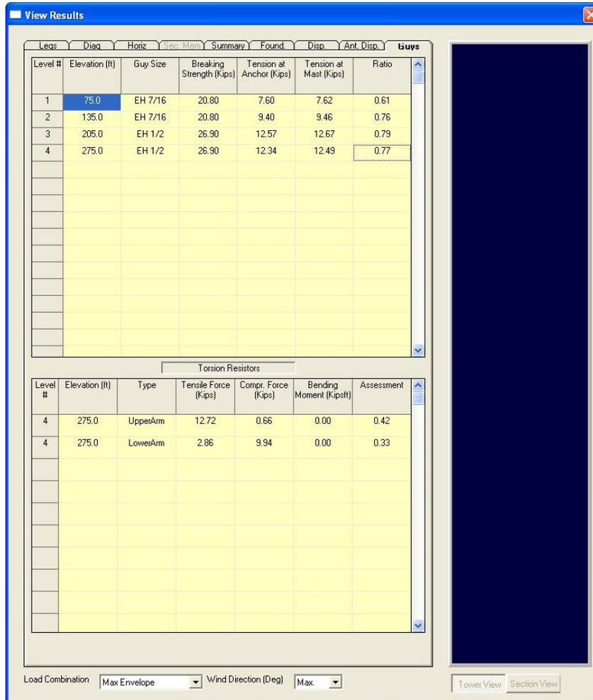
Also, on the bottom of the screen, the user may select the load combination for which results are to be displayed. Load combinations selected from the analysis menu are shown in the load combination list. Specific wind direction may be chosen or simply the envelope of the maximum values.
