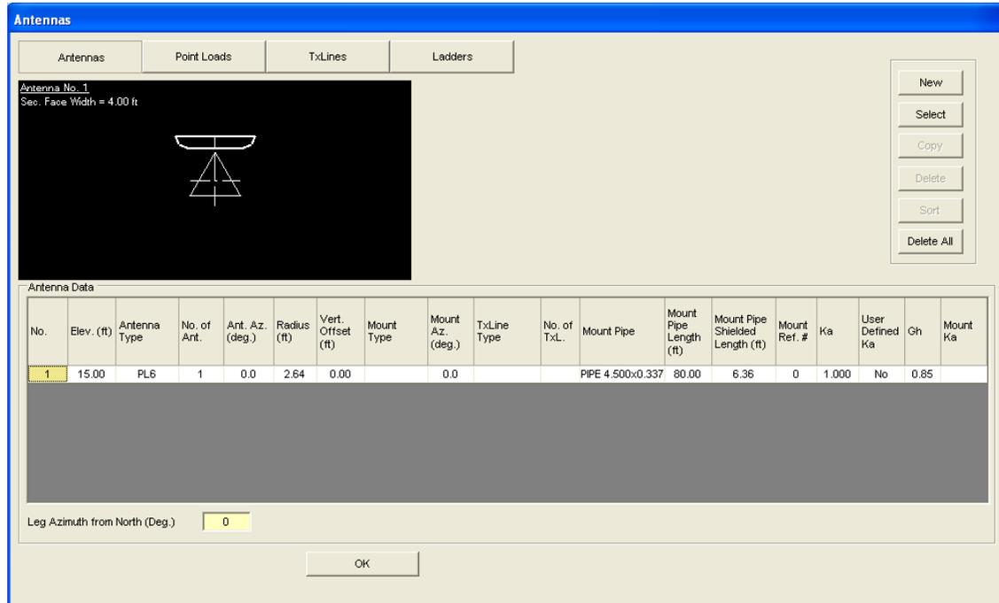
In this window the tower elevation is shown along with the plan cross-section at the marked antenna. To add a new antenna select **New** and a blank line with an antenna type (none) is shown. The user inputs the following data as defined below:
