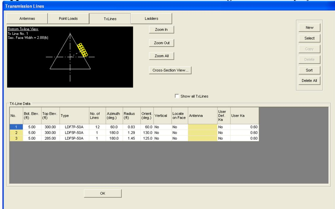
In this window the tower elevation is shown along with the tower cross-section at the bottom of the Tx-line. To add a new line or group of lines select **New** and a blank line with a line type (none) is shown. The user inputs the following data as defined below:
