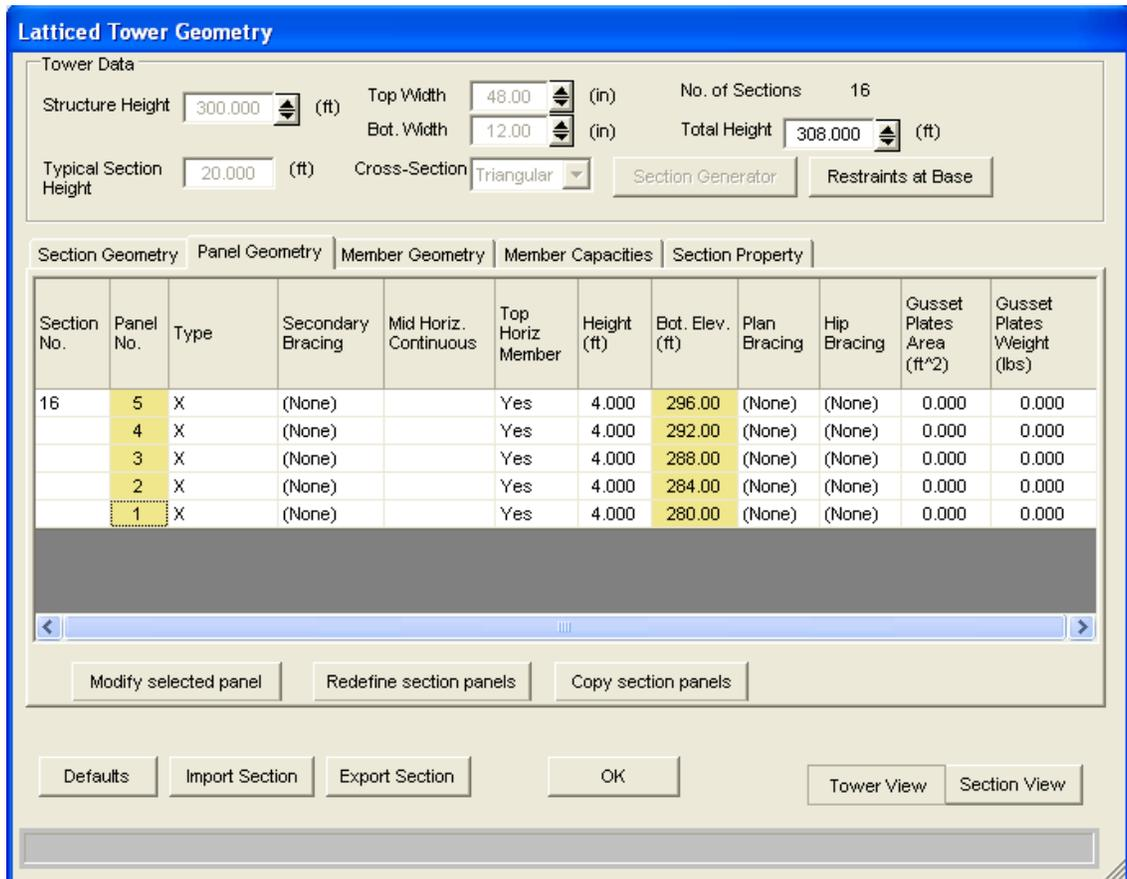
On the next Tab “Panel Geometry” the user can define the number, type, height of panels for the selected section. From the section column, other sections can be selected for Panel definition. Also on the same window the user can modify selected panels, change heights for different panels, redefine section panels and or copy section panels to other section(s).
