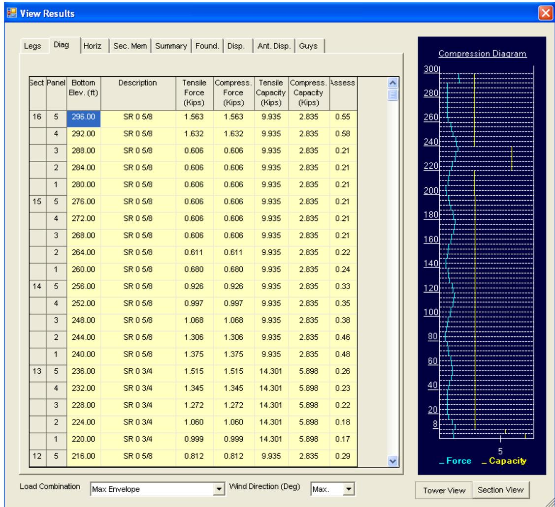
Also, on the bottom of the screen, the user may select the load combination for which results are to be displayed. Load combinations selected from the analysis menu are shown in the load combination list. Specific wind direction may be chosen or simply the envelope of the maximum values.
