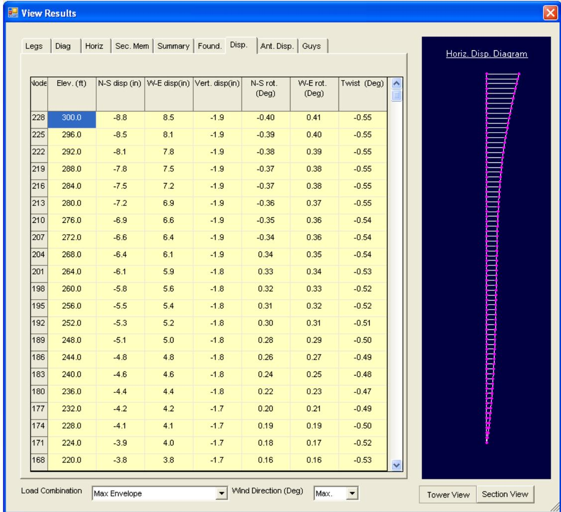
The displacements can also be viewed for the maximum envelope or any of the load combinations or wind directions.
